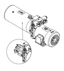
The W83A series power pack is designed for applications that need high pressure and larger flow,but use a low-power A.C. motor. The power pack uses a special manifold (W800553). All screw-in cartridge valves have been designed to be adjusted easily to service the power pack quickly. They still have the same dimensions and functions as the standard manifold (W800532).
